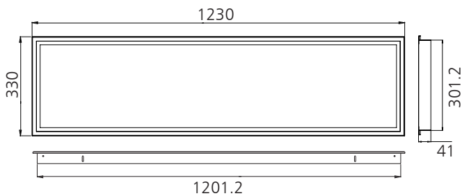
Model: UP-RF30120-01 Apply to led panel light 295x1195mm Ceiling kit size: 330x1230mm 310x1210mm cutout 1.175kg/pcs 5pcs/ctn Carton Size: 1300x330x400mm
